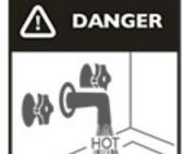
Water temperature over 125°f (52°c) can cause severe burns instantly resulting in severe injury or death.
