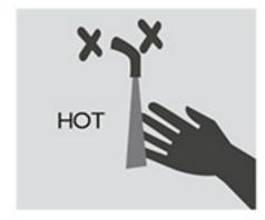
Water temperature over 125° F can cause severe burns instantly or death from scalds.
